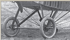
Undercarriage detail from Jeannin Stahltaube 283/14 (D). Note the dark painted wire wheels.
